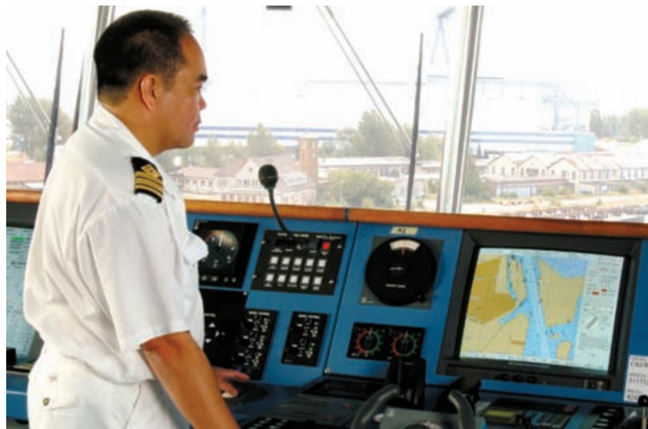
Electronic charts and ECDIS can make it easier to update folios, and may also reduce the burden on the navigator
